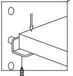
Adjust Leveler if needed to level case on uneven floor.
