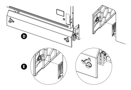
Open the fixing part on the Toe Kick(p). (D)
