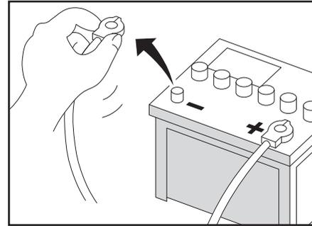
To avoid potential shorts in the electrical system, be sure to disconnect the (-) battery cable before installation. Use this unit with a 12-volt battery and negative grounding only. Failure to do so may result in a fire or malfunction.
