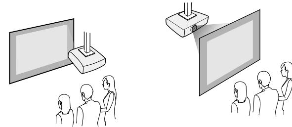
Select the correct **Projection** option in the projector's **Installation** menu according to the installation method being used. If necessary, turn on the **Inv Direction Button** setting in the projector's **Installation** menu and adjust the **Menu Rotation** setting in the projector's **Display** menu.
