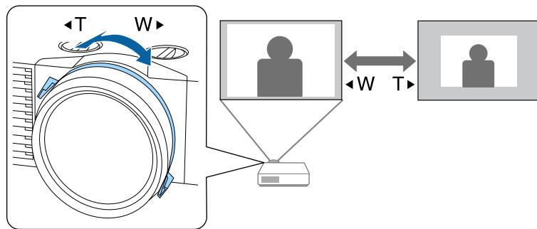
You can correct the focus using the focus ring. (EB-L890E/EB-L895E/EB-L690E/EB-L890U/EB-L790U/EB-L690U)
