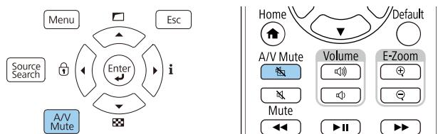
The light source turns off and the projected image and sound are interrupted.
