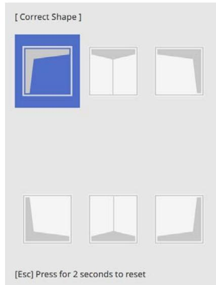
9 Press the arrow buttons to adjust the image shape of the selected area as necessary.
