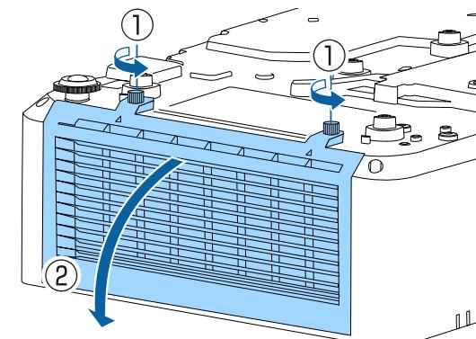
**5** Pull the air filter out of the projector.
