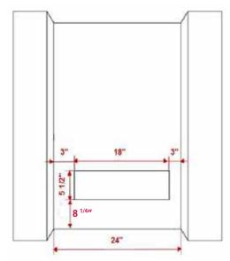
Required minimum air gap clearances: 1/4" sides
