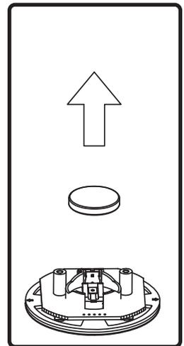
4. Install (1) CR2032 battery and reassemble the remote body.
