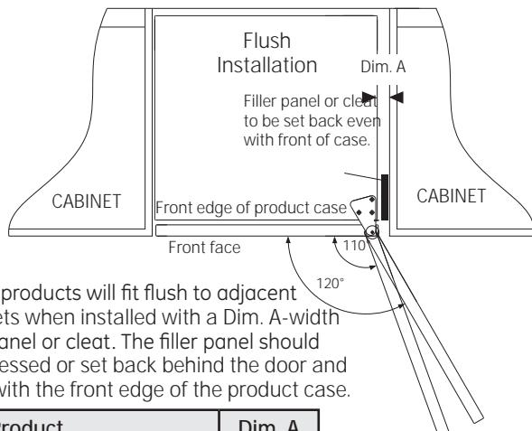
These products will fit flush to adjacent cabinets when installed with a Dim. A-width filler panel or cleat. The filler panel should be recessed or set back behind the door and even with the front edge of the product case.
