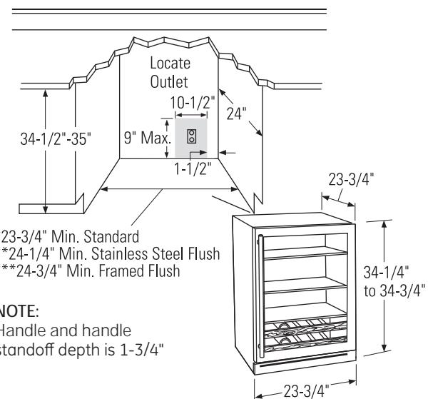
\*For a standard installation of Custom-Framed unit: The product must be installed so that the front face will project 2" forward of adjacent cabinets. This position will allow a full door swing and prevent interference with adjacent cabinetry. The opening between cabinets must be 23-3/4" minimum.
