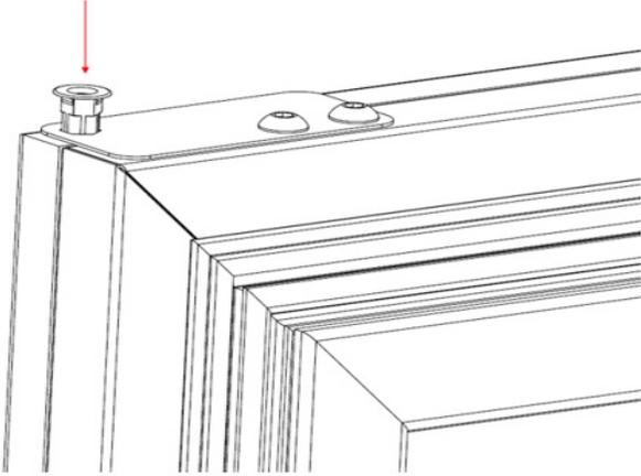
Align hinge bushing with top hinge and reinstall upper hinge pin using 1/8" Hex Key so that the pin is flush.
