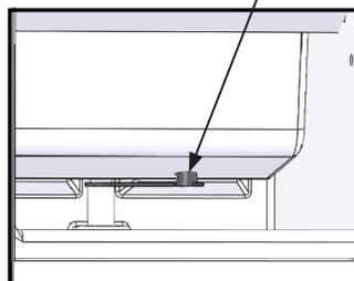
Pour cleaning solution slowly onto the front edge of evaporator plate behind the grid cutter.
