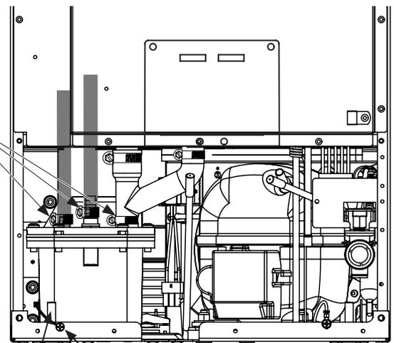
Drain pump ground wire connection
