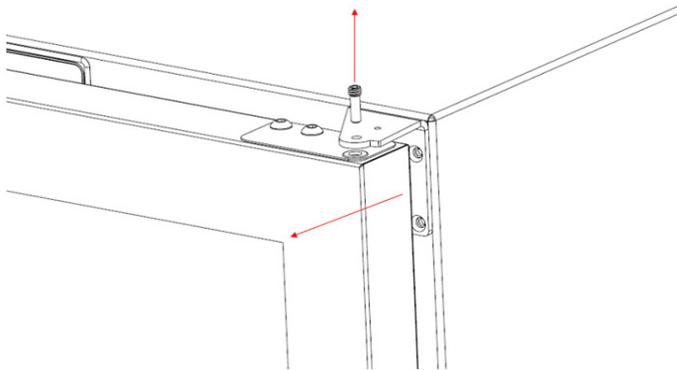
Remove the hinge bushing from the adaptor plate. A new bushing is included in the literature pack with your unit.
