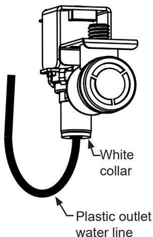
8. Reconnect the water valve outlet water line.
