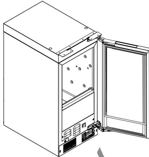
The light switch for changing the light color is located in the toe grille. Move the switch to the left or right to change the color of the light between blue, white, or amber.
