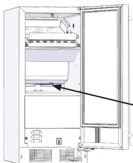
Remove the black reservoir drain plug from the bottom of the reservoir.
