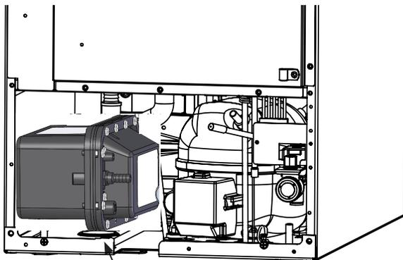
Rotate drain pump and remove from back of ice machine.
