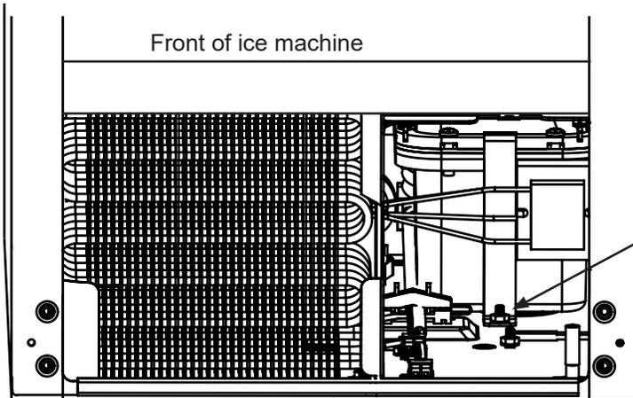
Remove the hex nut on front drain pump bracket with the  $\frac{3}{8}$ " socket then remove the bracket.
