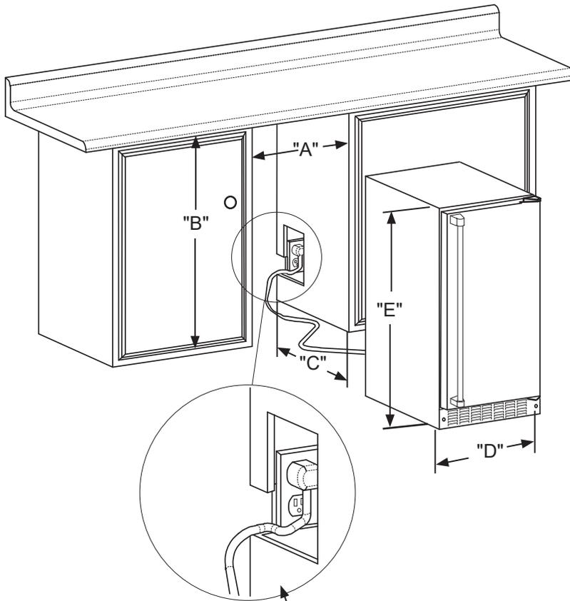
If necessary to gain clearance inside the rough-in opening a hole can be cut through the adjacent cabinet and the power cord routed through this hole to a power outlet. Another way to increase the available opening depth is to recess the power outlet into the rear wall to gain the thickness of the power cord plug. Not all recessed outlet boxes will work for this application as they are too narrow, but a recessed outlet box equivalent to Arlington #DVFR1W is recommended for this application.
