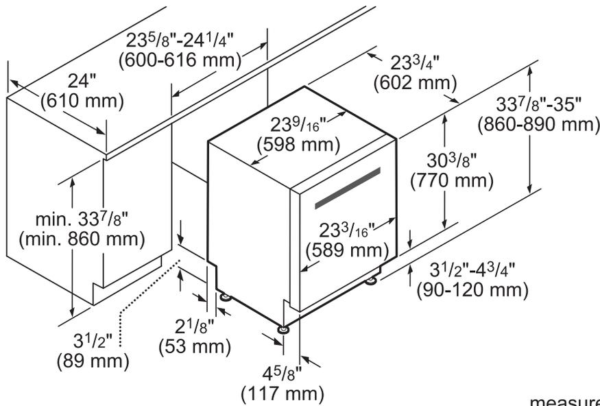
measurements in inches and mm
