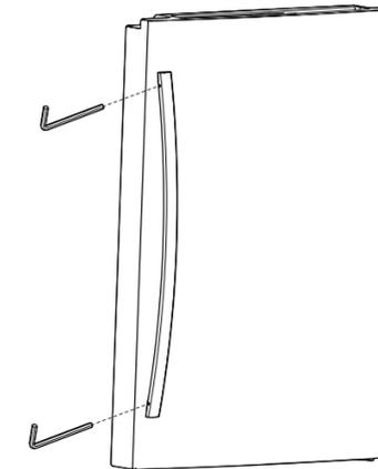
Tighten the screws at the top and bottom of the handle with the Allen wrench.
