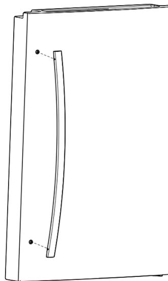
Place the handle over the mounts, ensuring the holes for the screws face the door opening.
