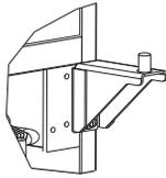
2. Remove corresponding screws on opposite side of cabinet. On some models there may be a nut behind one or both screws on either side.
