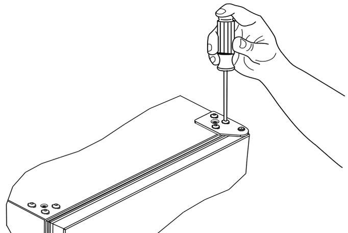
4. Remove door by tilting forward and lifting door off bottom hinge. Retain shoulder washers; they will be reused.
