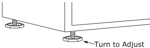
3. Confirm the unit is level after each adjustment and repeat the previous steps as needed.
