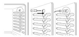
The meat probe icon flashes in the display if the meat probe is properly connected.
