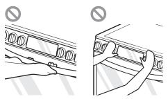
Do not push or pull the range by grabbing the open oven door or cooktop only. Doing so can result in serious damage to the range.
