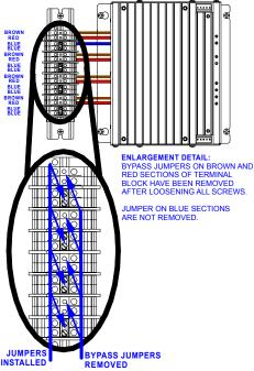
Wiring Diagram of the Terminal Block to the Module (Right Side Double-wide Enclosures)
