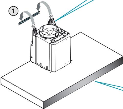
EN - Hood fastening (1), check valve installation and suction pipe assembly (3).
