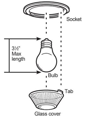
**⚠ CAUTION** Before replacing your oven light bulb, disconnect the electrical power to the range at the main fuse or circuit breaker panel. Be sure to let the light cover and bulb cool completely.
