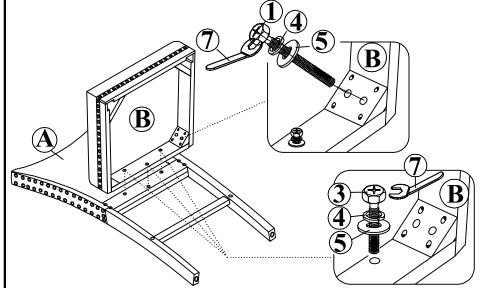
Step 1: Place the Chair Back (A) on the floor. Attach Seat Box w/Seat Cushion (B) Chair Back (A) by to inserting the Flat Washer (5), Lock Washer (4), Short Bolt (3) into the holes at the rear bar of the seat frame. Insert Flat Washer (5), Lock Washer (4), Long Bolt (1) into the holes at the corner block of the seat box. Tighten all Bolt with Open Wrench (7). Do not fully tighten.
