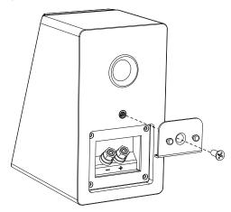
**5)** Connect the speaker wire to your binding posts and hang the Prime Elevation on the Multi-Angle Wall Bracket (patent pending) as shown. The foam gasket will make a tight fit and reduce any possible vibration noise.
