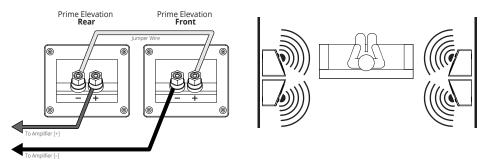
**Dipole Mode -** In dipole mode, one Elevation speaker is electrically reversed from the other, or "out of phase." This will provide a more diffuse and non-directional surround sound effect.
