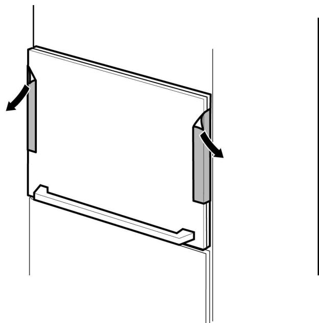
3. Remove styrofoam plates from backside of door.
