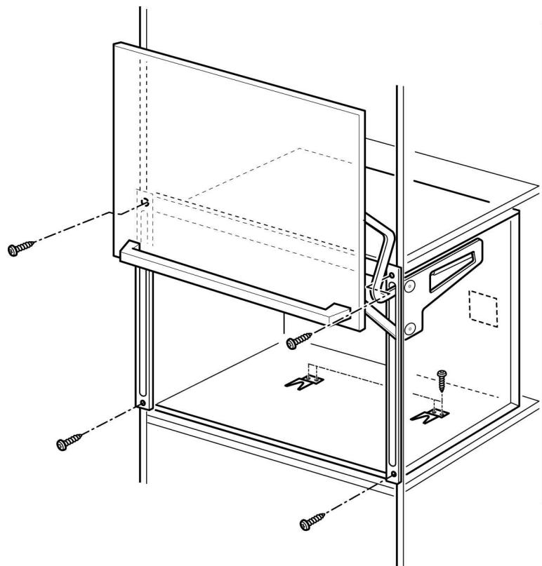
5. Optional: Slide in the Thermador microwave MBESLFTD in such a way that the fixing brackets engage the appliance feet.
