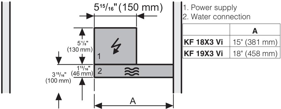
Install a pressure limiting device and water hammer arrester for inlet water pressures exceeding 80 psi. (Refer to Uniform Plumbing Code, Sections 608.2 and 609.10) Never install or operate where inlet water pressure may exceed 120 psi.
