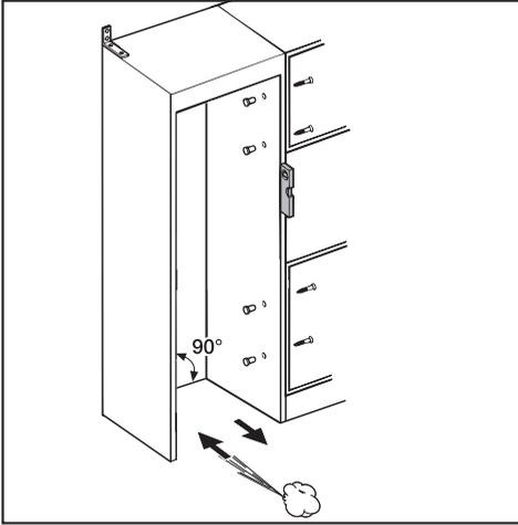
The housing unit must be carefully aligned using a spirit level before installing the appliance. The unit corners must be at right angles, as otherwise the furniture door will not align correctly with the 4 corners of the appliance.
