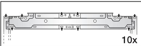
Please note: When attaching the mounting frame onto two adjacent doors (see "Front panel gap kit") screw into the thicker outer frames of the doors **only**.
