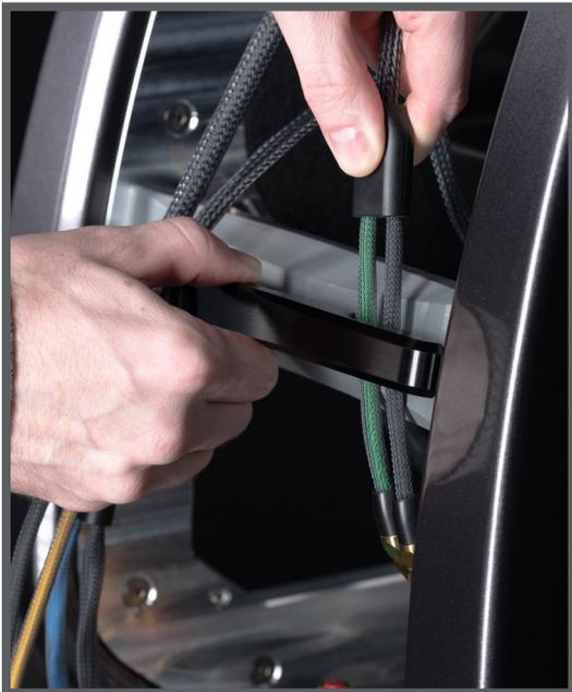
**Note: It is extremely important to ensure the adjustable cable clamps are tightened. Failing to tighten the clamp compromises the gas-tight seal of the module. Hand-tightened to “snug” is sufficient.**
