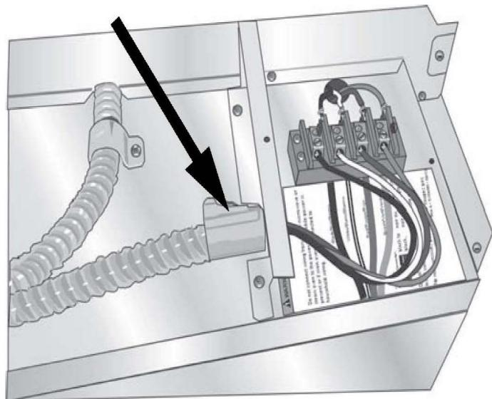
4. Snap the conduit connector into the hole by pressing it in until it clicks into place.
