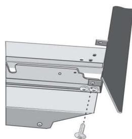
Align the outer flanges with the outside of the universal brackets. Fasten with one ( 1 ) screw each into the end hole of each universal bracket.
