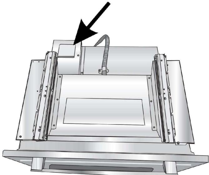
2. Remove the cap from the conduit access hole in the side of the oven-mounted junction box.
