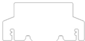
Restrictor plate for Set 1, Set 2 (Part # 761-060F)
