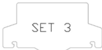
Restrictor plate for Set 3 (Part # 761-143F)
