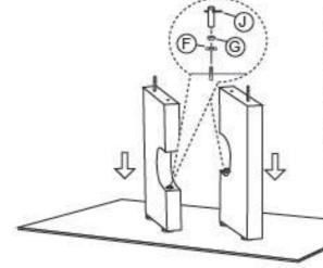
2. Secondly, make the long rods (D) and short rods (E) pass through the side boards (C) and use the tooling (J) tighten the metal gaskets (F) and the small bolts (G) as picture.
