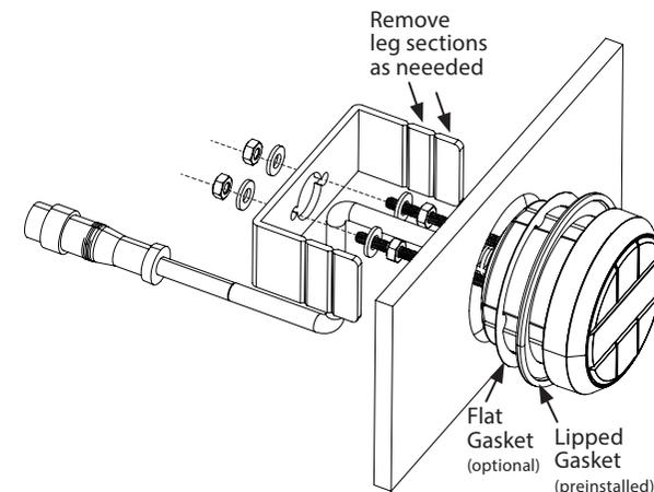
4. Install a nut and washer near the middle section of each stud (see diagram) and place the MMR-20-BE into the mounting hole.
