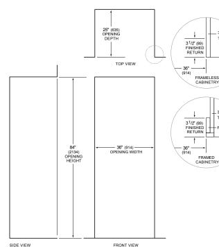
NOTE: 31/2" (89) finished returns will be visible and should be finished to match cabinetry
