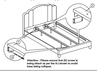
STEP 5: Tighten all the 4 corner, follow by assembly of the slat holders with LVL slats as shown.
