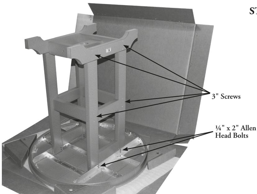
**STEP #3 -** First fasten the Second Base to the Aluminum Frame of the Top using 4- 1/4" x 2" Allen Head Bolts and 4- 1/4" Flange Nuts. Second fasten the Footrests and Cross Support to the Base using 3" Screws.
