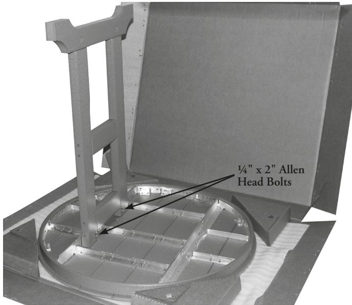
**STEP #1 -** Fasten one Base to the Aluminum Frame of the Top using 4- 1/4" x 2" Allen Head Bolts and 4- 1/4" Flange Nuts.
