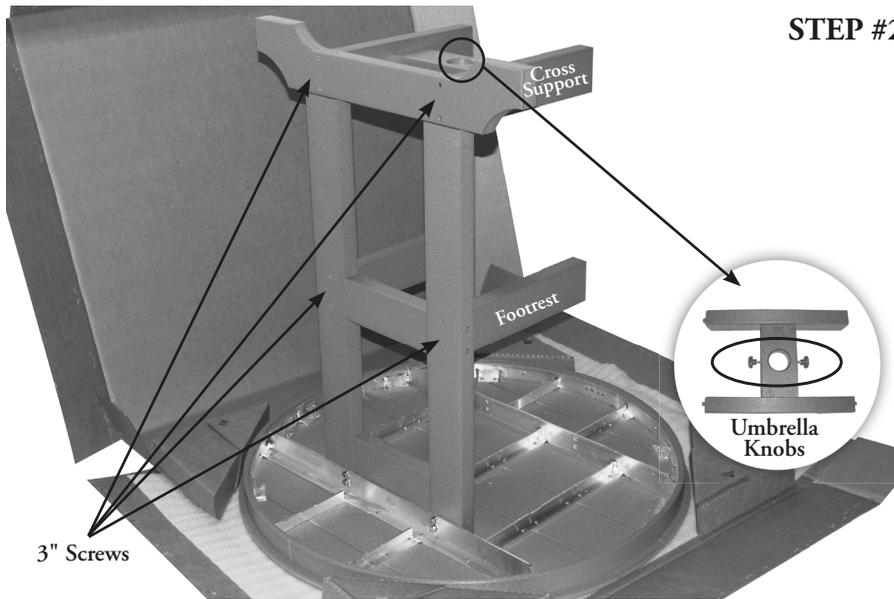
**STEP #2 -** First attach the Cross Support to the Base using 3" screws. Second attach the two Footrests to the Base using 3" screws (counter and bar height only).
