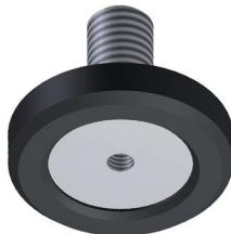
With great care turn the cabinet the right way up. Place the cabinet in the desired location, checking that it is level on all sides. If slightly off-level, unscrew the foot at the lowest point and check again. Continue this process until the cabinet is fully level. Use the locking nuts (illustrated on page 3) on each foot to fix the feet in place and to stop any unwanted vibrations.
