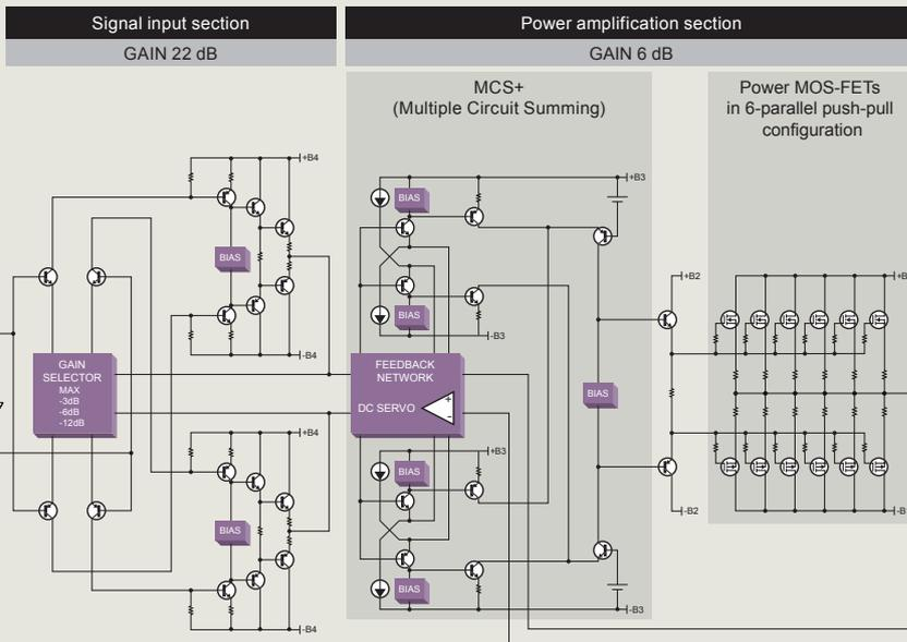
■ Circuit diagram of amplifier section (one channel)
