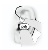
To know whether the earphone tip is properly sealed within your ear, insert the earphone tip into the ear canal and try listening to ambient noises with no music playing. If there is a proper seal, the sound will be dull and distant. If the sound is clear, the earphone tip is not properly sealed inside the ear. If the sound can faintly be heard in the distance but pressure is felt inside the ear, the earphone tip has been over-inserted and must be readjusted.
