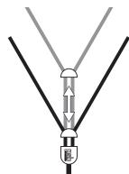
Move the adjustment slider up or down to reduce or increase the amount of loose cord between the left and right earpiece.
