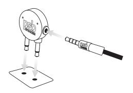
Use the standard cable and the supplied dual 3.5mm airline adapter to connect to in-flight entertainment systems equipped with dual output connectors.
