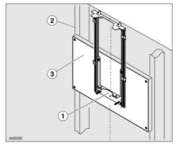
Determine and mark the location of the retaining plate ① for the canopy as outlined on the "Installation diagram".
