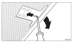
If the filters have been installed incorrectly, you can insert a small screwdriver into the slit to disengage the locking clip.
