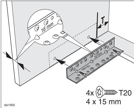
The runners are made for side walls of 5/8" (16 mm) and 3/4" (19 mm). Screw on the angled side which has the imprint of the respective cabinet wall measure.
