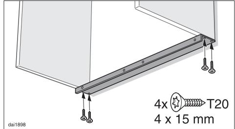
■ Screw the space bar flush with the wall under the cabinet side walls.
