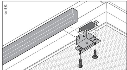
The installation kit DML 400 is necessary. It can be obtained as an optional accessory from Miele. The installation kit has an installation manual supplied.
