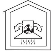
Air is drawn through the grease filters and an **active charcoal filter**. The filtered air is then recirculated back into the kitchen.
