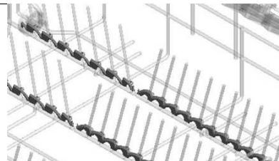
Supports for cups and long objects (ladles, spoons, etc.), in the rear; can be tipped to the vertical position when not in use.
