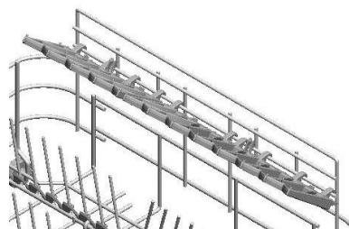
**Wine pro.** Support for long-stem glasses. When lifted out of the stowed position (0) it snaps into three different positions (1-2-3).
