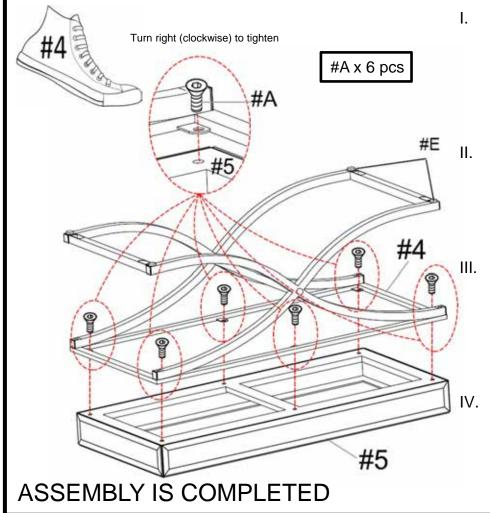
With the help of another person, carefully place the table top (#5) facing down on a protected surface. Align the brackets of the assembled table frame (#4) with the pre-drilled holes on the table top (#5).
