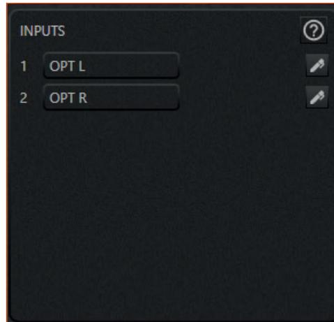
**Remark:** for digital input channels sensitivity should not be adjusted.
