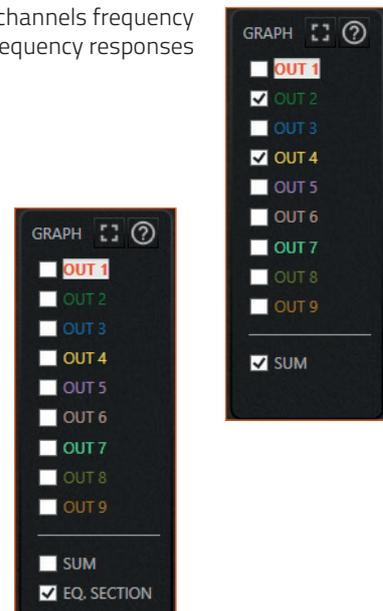
If the parametric equalizer is used, the EQ. SECTION item appears at the bottom of the graph settings panel: putting the check mark on it, a dashed line that represents the frequency response of the equalizer selected section, is shown on the graph.
