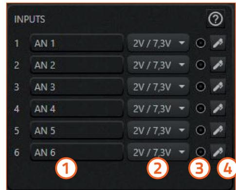
The image below shows the sensitivity scale for an analog input channel: the value at the top indicates the lowest sensitivity level; the value at the bottom corresponds to the highest sensitivity level. The scale has double values: they are related to the type of analog input connector used, i.e. SPEAKER IN or PRE IN.
