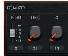
**WARNING:** when changing from the parametric type to the graphic type, some set parameters can be modified according to the constraints imposed by the graphic equalizer (filter type, frequency, form factor (Q), ...).
