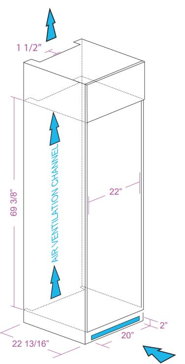
Your XO Wine Cabinet must be vented to operate properly. Air enters below the cabinet in the front, passes up behind the unit and exits at the top.
