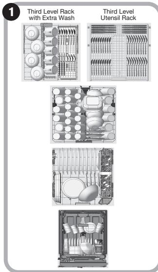
**Prepare and Load the Dishwasher** (Up to 16 Place Setting Recommended Loading Pattern)
