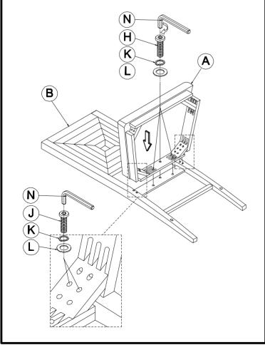
STEP 2: Do not fully tighten the screws
