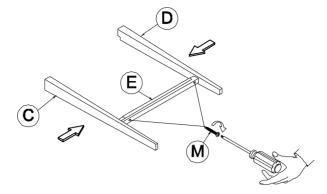
STEP 4: Using the Allen Key to tighten all bolts
