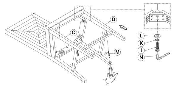
STEP 5: Using the Philips Head Screw driver to tighten all screws
