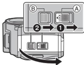
2 **Battery**: Being careful about the battery orientation, insert all the way until you hear a locking sound and then check that it is locked by lever (C). Pull the lever (C) in the direction of the arrow to remove the battery.
