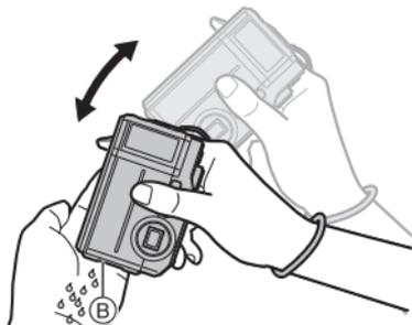
**3 Dry the camera by standing it on a dry cloth in a well ventilated shaded area.**
