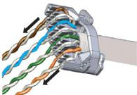
c. Ensure that each wire lies below the top surface of the termination module as indicated by the dashed line in the illustration below.
