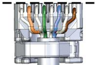
8. Trim the wire pairs so that they are flush with the edge of the channels.
