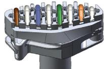
9. Trim the excess DM-CBL-ULTRA braid shield or the excess DM-CBL-8G drain wire and foil shield.
