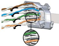
b. Fully seat each wire into the appropriate channel.
