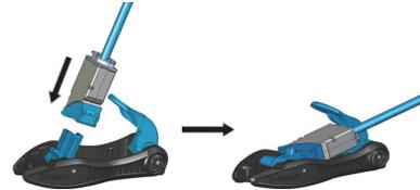
3. Ensure that the DM-CONN-ULTRA-RECP is seated properly in the termination tool, and then fully depress the lever until a click is heard—do not partially depress the lever and then lift the lever to reseat the DM-CONN-ULTRA-RECP.
