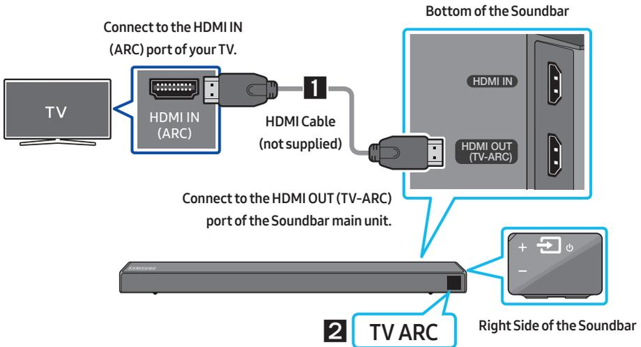
1. With the Soundbar and TV turned on, connect the HDMI cable (not supplied) as shown in the figure.
