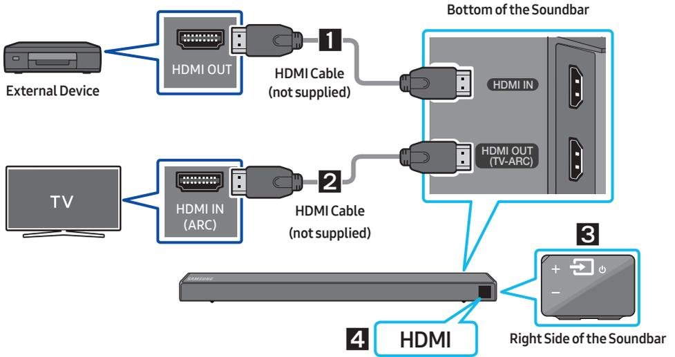
1. Connect an HDMI cable (not supplied) from the **HDMI IN** jack on the back of the product to the **HDMI OUT** jack on your digital device.
