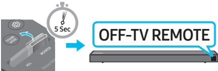
3. If you want to control the Soundbar with your TV's remote, push up and hold the **WOOFER** button for 5 seconds repeatedly until "**ALL-TV REMOTE**" appears in the display. Then, use your TV's menu to select external speakers.
