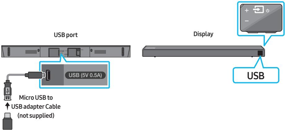
1. Connect a Micro USB to USB adapter cable with a male USB 2.0 Micro USB plug (Type B) on one end and a standard female 2.0 USB jack (Type A) on the other end to the micro USB jack on your Soundbar.
