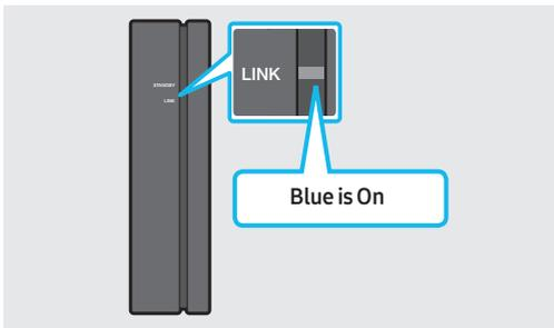
The LINK LED indicator stops blinking and glows a solid blue when a connection is established between the Soundbar and the Wireless Receiver Module.
