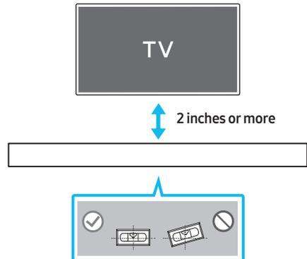
2. Align the **Wall Mount Guide's Center Line** with the center of your TV (if you are mounting the Soundbar below your TV), and then fix the **Wall Mount Guide** to the wall using tape.
