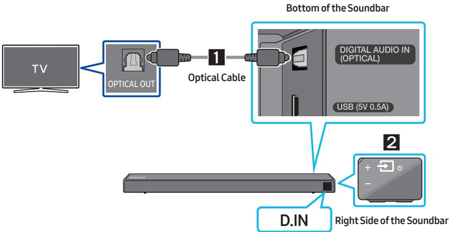
1. Connect the **DIGITAL AUDIO IN (OPTICAL)** jack on the Soundbar to the **OPTICAL OUT** jack of the TV with a digital optical cable.
