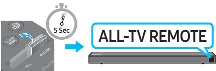
4. If you want to return the Soundbar to the default mode (control by a Samsung TV remote), push up and hold the **WOOFER** button for 5 seconds repeatedly until "**SAMSUNG-TV REMOTE**" appears in the display.
