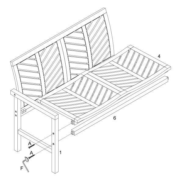
Use Bolt (A), Hex Key (F) to secure part (1) to seat panel (4), secure part (1) to part (6).
