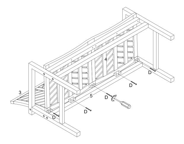
Use screw (D) and a screwdriver to secure seating panel (4) to support bar (5).
