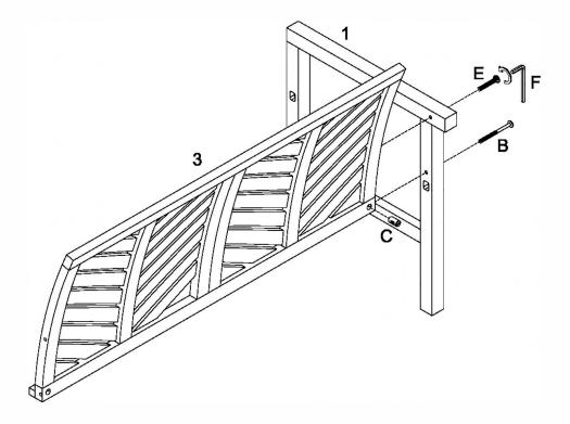
Insert (C) into Part(3), use bolt (E), (B) and Hex Key(F) to secure Part (1) to Back Panel (3).
