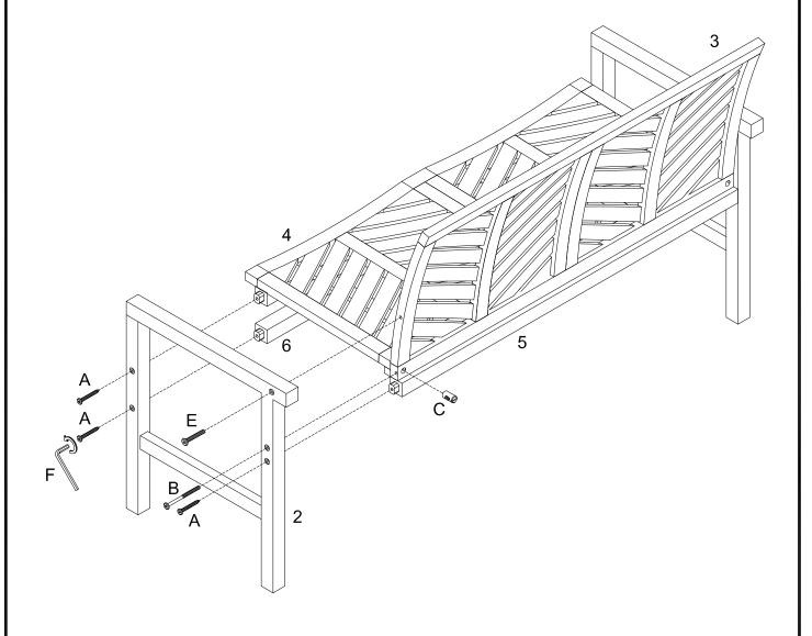
Insert part (C) to part (3),use Bolt (A), (B), (E), Hex Key (F) to secure Part (2) to back panel (3), seat panel (4) and part (6).
