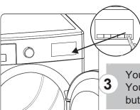
You can select additional functions for drying. You can run the program by pushing Start / Pause button.
