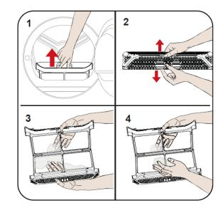
After the dryer has been used for a certain period of time, if you encounter a layer that will cause an obstruction on the filter surface, wash the filter with warm water to clean the layer. Dry the filter thoroughly before reinstalling it again.
