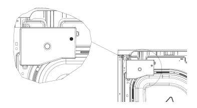
2. Remove the clamp of the strain relief which has already been attached on your machine. Then pass the clamp through the supply cord and put the supply cord through the main body of the strain relief. Be sure that wire insulation of the cord inside the strain relief.
