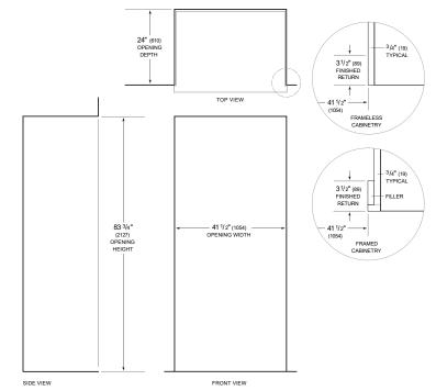
NOTE: 3<sup>1</sup>/2<sup>\*</sup> (89) finished returns will be visible and should be finished to match cabinetry Shaded line represents profile of unit.
