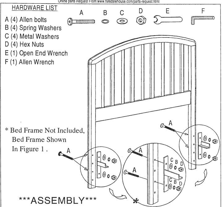
Attach each Bed Frame (\* Not Included) to posts on Headboard, using 2 Allen Bolts (A), 2 Metal Washers (C), 2 Spring Washers (B)& 2 Hex Nuts (D) per each side. Only Hand Tighten bolts & Nuts using Allen Wrench & Open End Wrench (E&F) once bolt bed frames have been attached. See Figure above for illustrated details.
