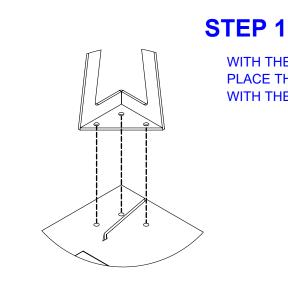
WITH THE HELP OF SOMEONE ELSE, PLACE THE METAL LEG ALIGNING IT WITH THE HOLES AT THE TOP.
