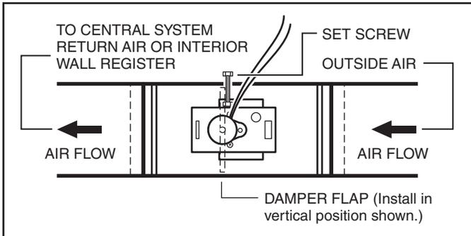
Install the damper as shown. Make sure damper flap is in a vertical position when closed and power is off. The set screw can be used to adjust the damper opening - thereby balancing the inside and outside air pressure when the range hood exhausts at high speed.
