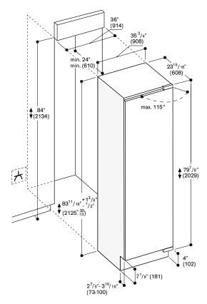
The door face dimensions are designed for a maximum gap of % " (3 mm). See more details on page 252.
