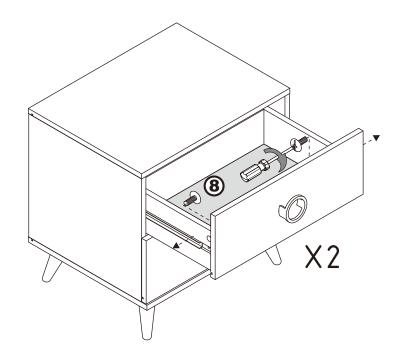
Extend the two outer slides of the runners so that they could align with the sides of the drawer.
