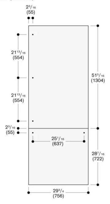
The door panel thickness is 3/4" (19 mm)
